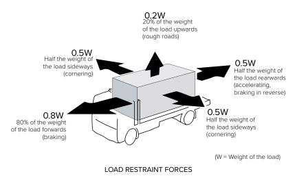
Note that these forces, and the forces that any load restraint system must be designed to meet or exceed, are equivalent to a low-speed collision between a heavy and light vehicle. That is, **any load restraint system for goods in/on a heavy vehicle or in a freight container must be capable of sustaining a low-speed collision between a heavy and light vehicle**.
